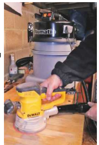
▲ A simple tapered adapter is supplied for power tools
